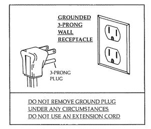
For your safety and protection, the Kenmore freezer is equipped with a special three-terminal type grounding plug on the electrical cord. It must be plugged into its own properly grounded three-prong outlet-115 volt, 60 Hertz, protected with a 15 amp time delay fuse or circuit breaker.
